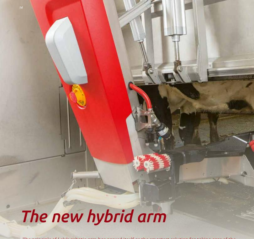
The principle of Lely's robotic arm has proved itself as the smartest solution for taking care of the milking process. It is underneath the cow during the whole milking process and reacts fast when a teat cup drops off to keep it clean. The arm follows the cow, allowing her maximum freedom of movement in the box.
